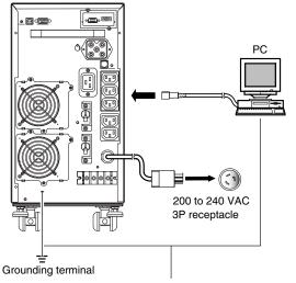
Connect the ground wire to the Grounding terminal.
